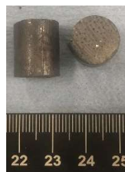
Left: S5 Ø13.5x18 mm cylinder Right: S5 in drill bit after tripped out of well.
