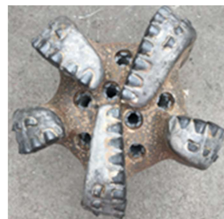
Left: S5 Ø13.5x18 mm cylinder Right: S5 in drill bit after tripped out of well.
